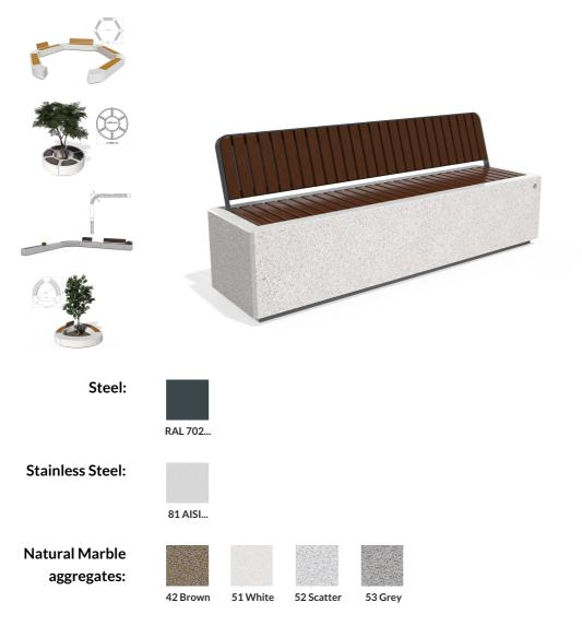
Bench model \*\*268-B\*\* is made from high-strength fiber-reinforced concrete with a homogeneous aggregate structure of natural marble or granite stones. The structural aggregates have a strictly defined size and color range, determining the main textures: white, scatter, gray, or brown. Various technological methods of treating the concrete surface ...
